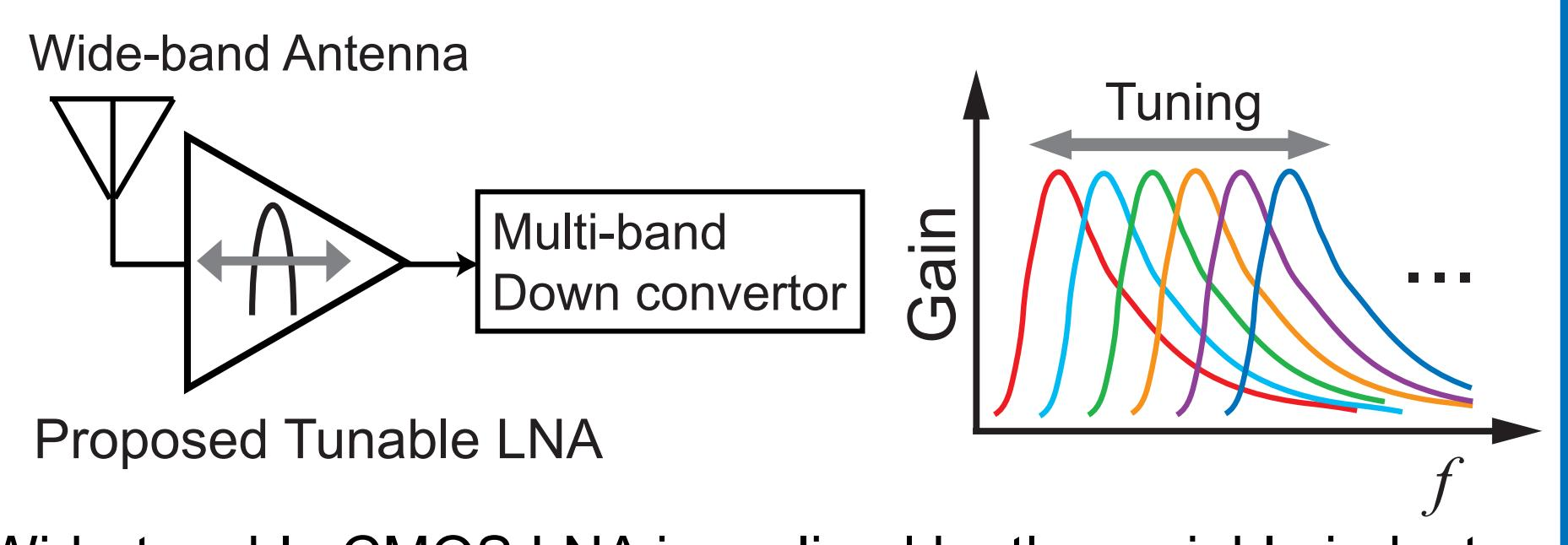
The proposed LNA achieves wide-tuning range with narrow-band gain and can be used for reconfigurable RF front-end.
