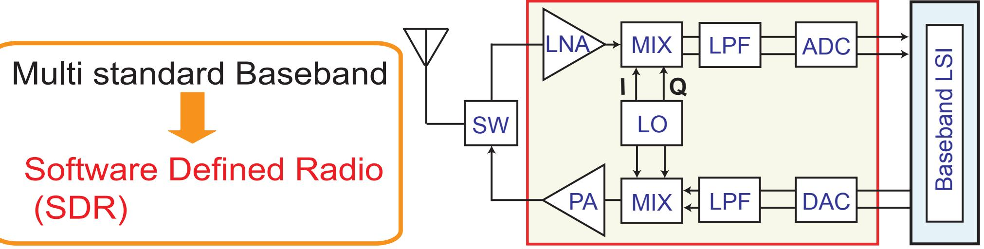
It is necessary for global roaming using SDR to realize Multi-band RF front-end
