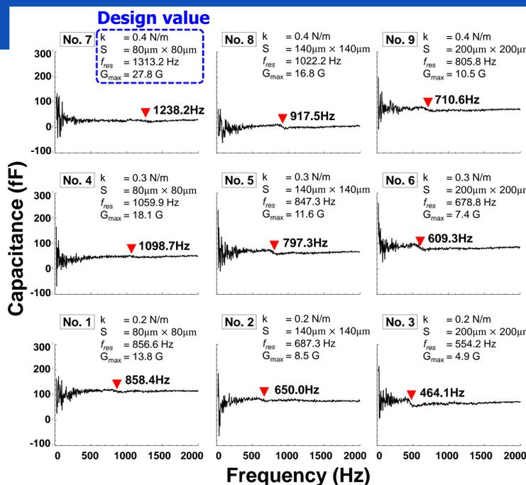
Measured capacitance as a function of sensing signal frequency
