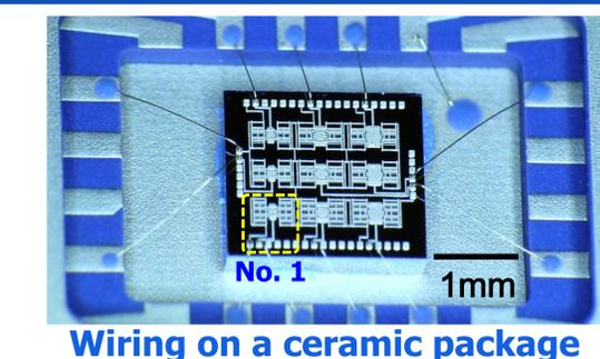
Wiring on a ceramic package
