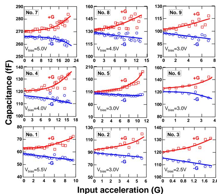
Measured capacitance as a function of input acceleration
