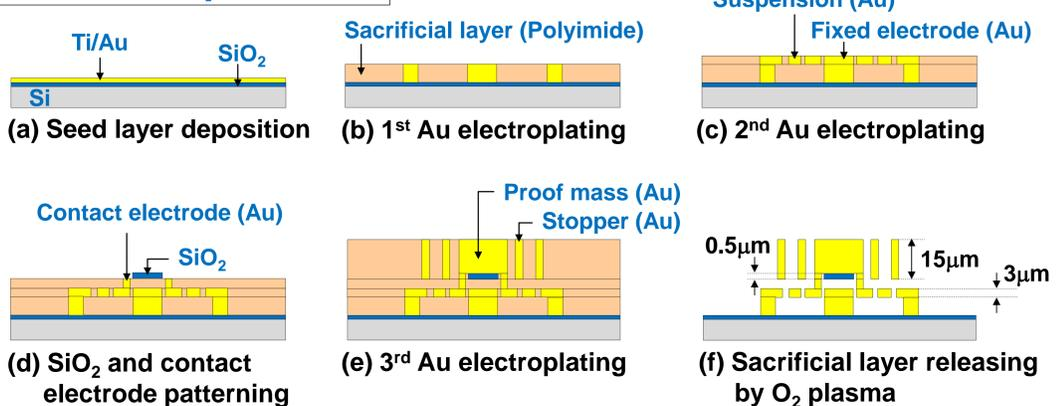
Microfabrication process for post-CMOS integration
