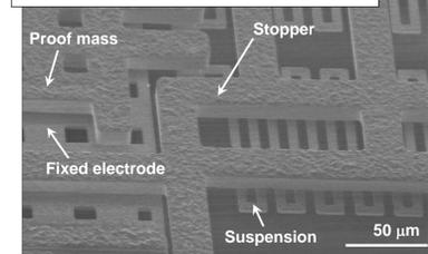
SEM images of the developed 3-by-3 MEMS accelerometer
